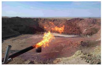
SHYRAK-1 WELL GAS FLARING DURING DRILLING
