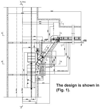
Fig. 1 Layout of the mechanical equipment of the batching chamber with the reinforced concrete hopper according to a new variant (section on the chamber).
