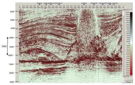
Figure. 4 Structure of Kobylandy. Inline 2552 seismic section showing deposition of the Middle Devonian complex
