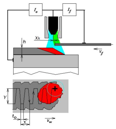
Fig. 1. Diagram of the plasma-arc surfacing process with transverse oscillations of the welding torch [1]: IO is the current of the main arc, and If is the current of the additional arc, vw is the rotation speed of the workpiece, vf is the flow of the surfacing alloy,  $\tau$  is the period, Y is the amplitude and to there is a form of transverse vibrations, Xk of the drop on the wire relative to the axis of the plasma torch on the wire feed speed, hare the height of the deposited layer.
