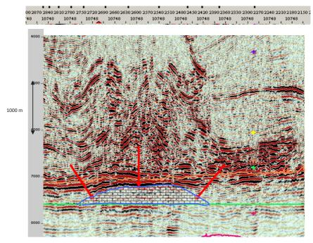
Figure 3. The structure of Kobylandy. Crossline 10652 seismic section showing prospective reef construction
