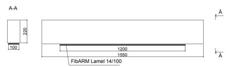
Fig. 3 — Reinforcement structure of the reinforced concrete beam with FibARM Lamel 14/100
