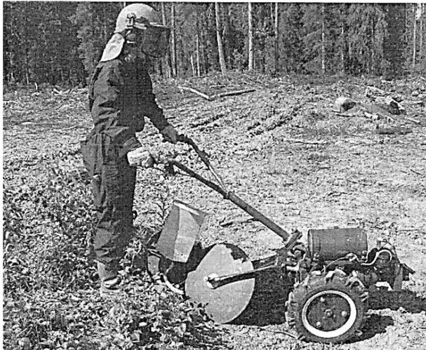
*Fig. 6. An experimental sowing unit based on a motoblock*
