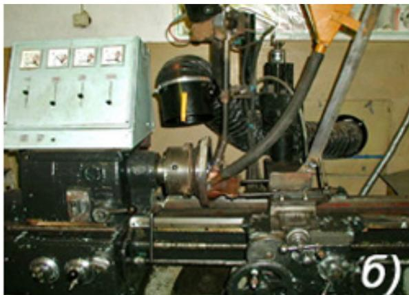
*Fig. 5. The surfacing labyrinth ring (a) and installation for surfacing parts such as bodies of rotation (b)*
