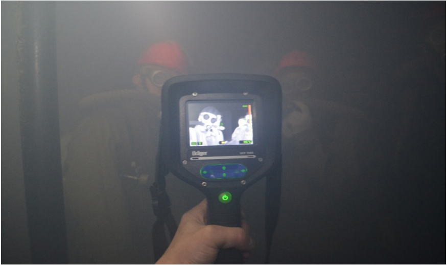
Fig. 3. Training in a respirator in a smoky workout. Monitoring the operation of a subgroup using a portable explosion-proof thermal imager
