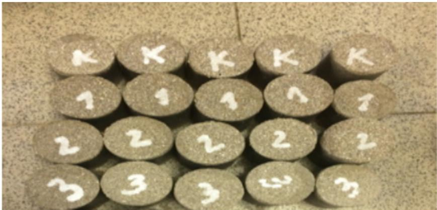
After getting samples of sand-lime brick and autoclaved treatment, technical indicators are constructed according to GOST 379-2015.
