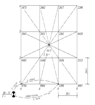
Figure 1 - Scheme of leveling with samples
