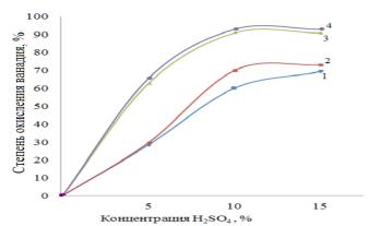
Figure 2 - Dependence of the degree of oxidation of vanadium on the concentration of electrolyte: 1 - raw ore of the Balasauskandyk deposit; 2 - raw ore of Kurumsak deposit; 3 - burnt ore (stub) of the Balasauskandyk deposit; 4 - annealed ore of Kurumsak deposit
