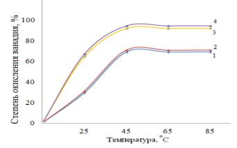
Figure 1 - Dependence of the degree of vanadium oxidation on temperature during electrooxidation: 1 - raw ore of the Balasauskandyk deposit; 2 - raw ore of Kurumsak deposit; 3 - burnt ore (stub) of the Balasauskandyk deposit; 4 - annealed ore of Kurumsak deposit
