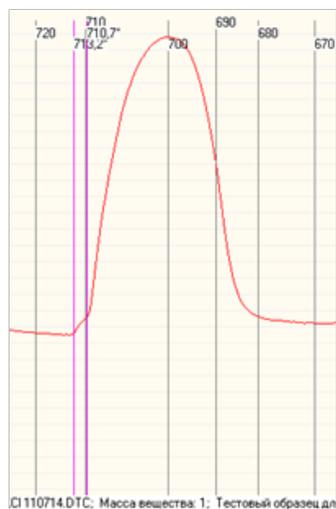
**Fig.2** Thermal curve of cooling system 20% LiF - 80% KCl
