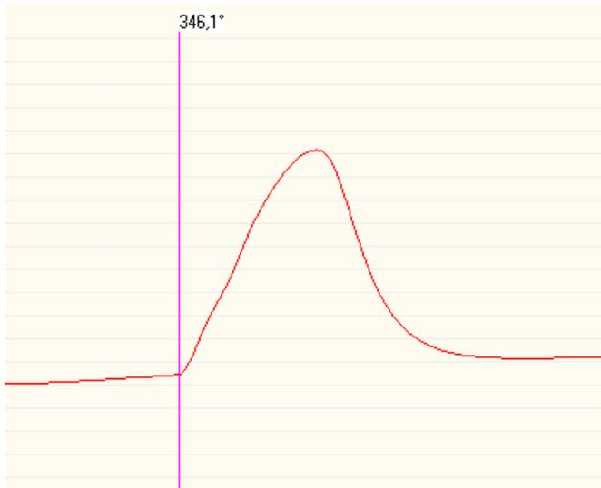
**Fig.6.** Thermogram of crystallization of 56LiCl-3,5 LiF-40,5 KCl (EQ.%)
