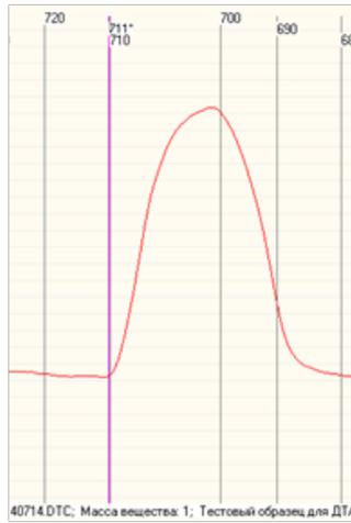
**Fig.3** Thermal cooling curve 19% LiF - 81% KCl
