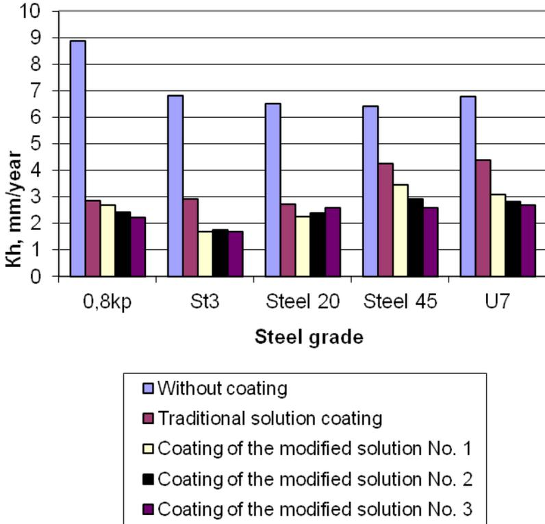
*Fig. 2. Comparison of the deep corrosion index of samples*
