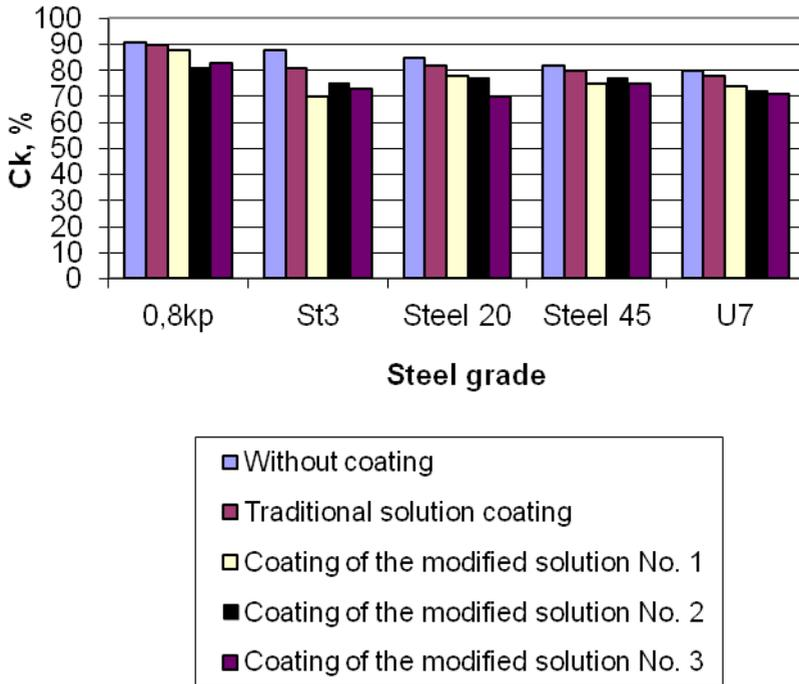
*Fig. 3. Comparison of the degree of cathodic control*
