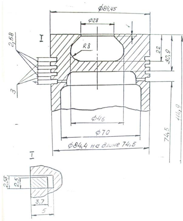
Fig.3. Sketch of piston and piston ring
