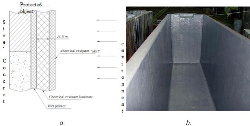
**Fig.2.** a. - the scheme of protecting laminate system,
