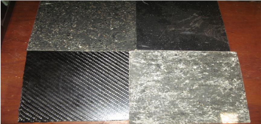
*Fig. 6. Samples of composite tiles from different fillers*
