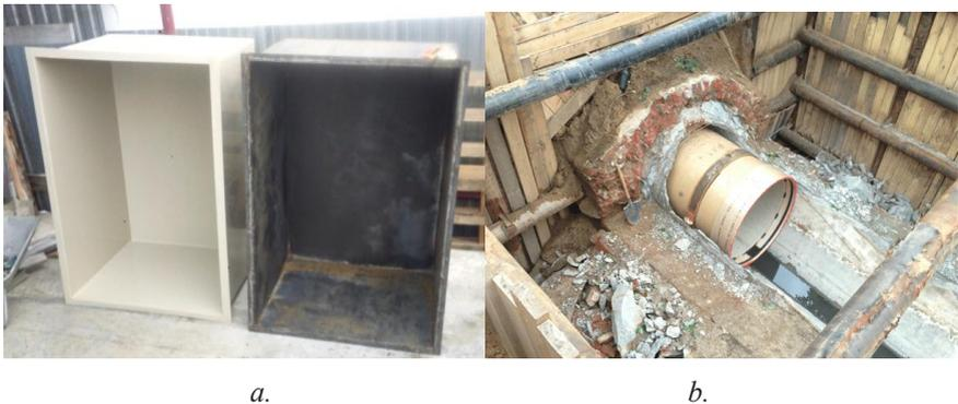
**Fig. 8.** a. – metal etching bath and polymer chemical-resistant insert,
