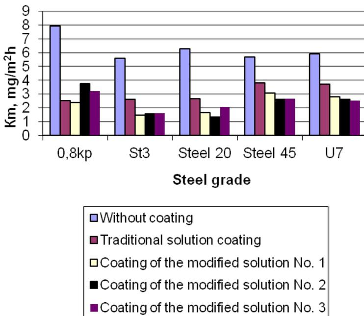
*Fig. 1. Comparison of the negative index of change in the mass of samples*
