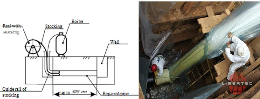
a. *Fig. 9. a. – scheme of installation of CIPP,*
