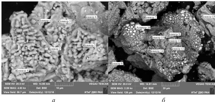
**Fig. 4.** Spectral analysis of titanium carbide samples: *a* - at 50 μm, taken from the laminar gas motion region; *b* - at 20 microns, selected from the turbulent region
