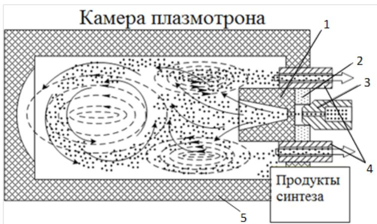
*Fig. 1. Scheme of the process of plasma-chemical synthesis: where, 1 is the nozzle, 2 is the dielectric ring, 3 is the electrode, 4 are the tubes for discharging the gas-vapor phase and finely dispersed residues*
