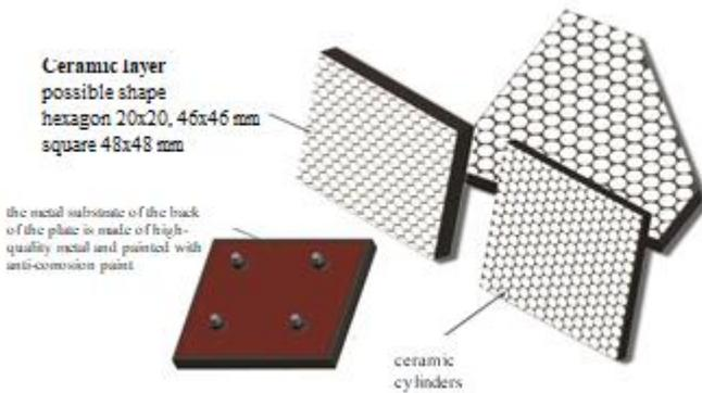
*Fig.11. Elements of rubber-ceramic lining*
