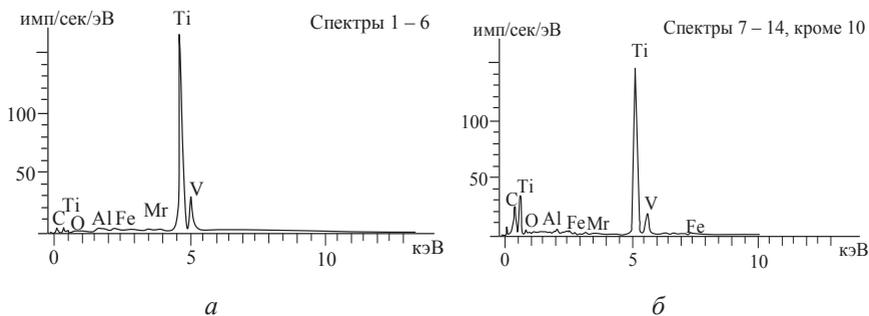
**Fig. 5.** Spectrogram of TiC samples: *a* - spectrogram from the 1st to the 6th mark, *b* - spectrogram from the 7th to the 14th mark, except 10
