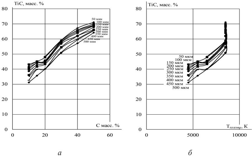
**Fig. 2.** Dependences of the change in the mass of TiC in the products of synthesis: *a* - on the mass of the carburizer C in mass. %; *b* - from the temperature of the plasma stream  $T_{\text{plasma}}$ , K
