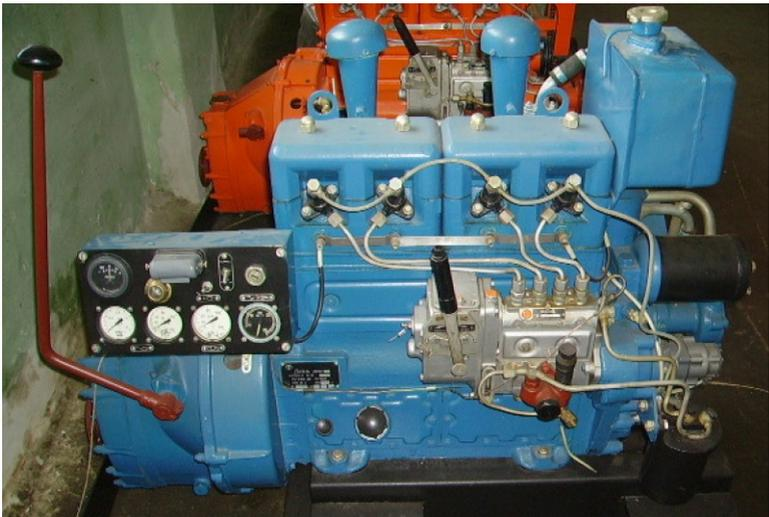
*Figure 1. Diesel 4ЧCIП 8,5/11 with reverse gear*
