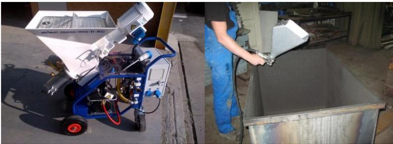
*Fig.3. a. - putty aggregate, b. – putty gun.*
